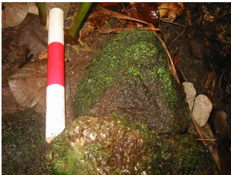
Figure 4. Survey control point engraved in stone and depicted on map (Podmore 1915). The scale is marked in 10 cm increments.
